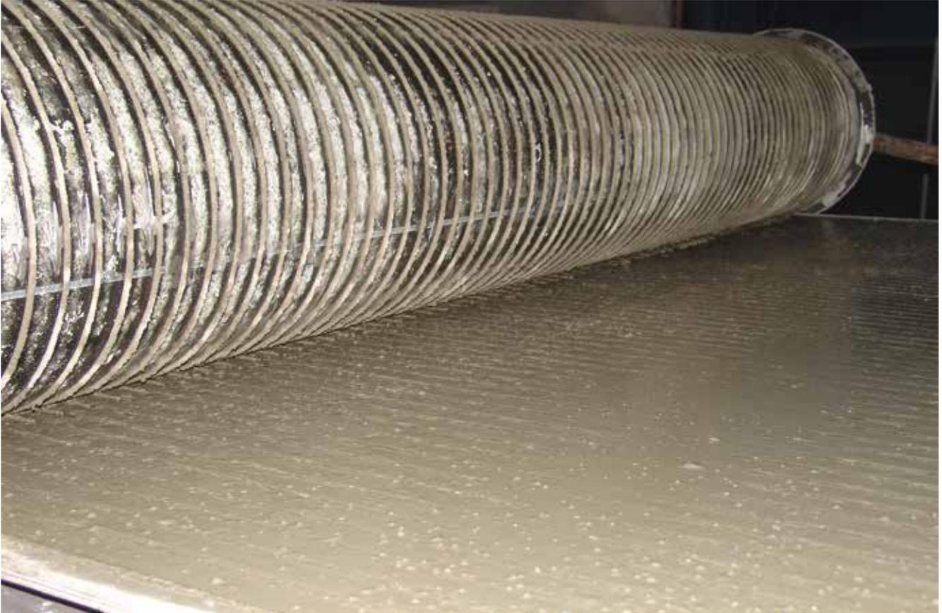
Dobashin developed this drum for texturing the double-tee slabs. He found the information he needed on the internet. **Courtesy of Leo Abramovich and Building Design International.**
